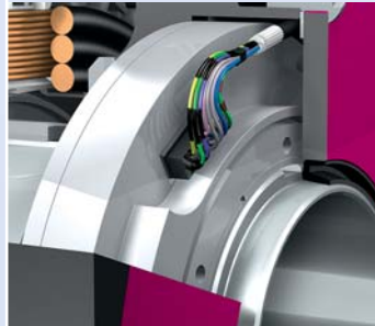
An EnDat® absolute encoder is used for the feedback system
