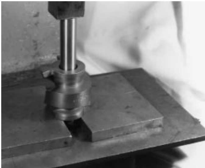
Fig. 6 Pressing out camshaft
