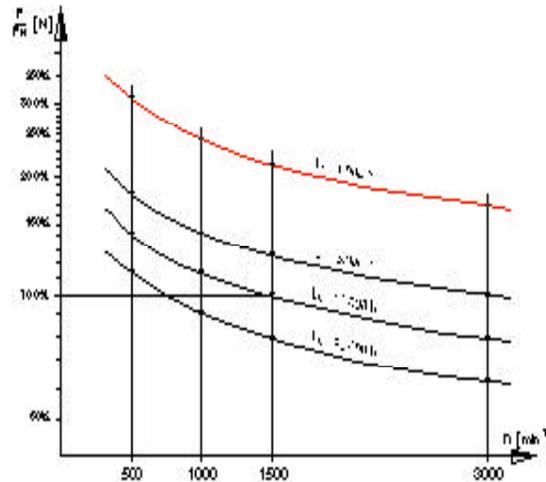
The value  $F_N$  refers to the load at the middle of the shaft, distance  $L/2$ . It is based on a service life of 10,000 h and a speed of 1500 rpm. For other speed and service life values,  $F_N$  can be calculated with the aid of the graph shown above. If additional axial forces occur, a recalculation of the bearing load should be performed by the factory.
