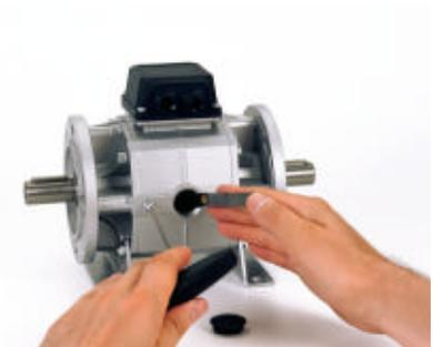
When the Combibox has reached maximum wear, the wear parts must be replaced. Wear parts include the brake magnet, the armature, and the clutch rotor. To order spare parts, provide the 11 digit part number, or the following information:
